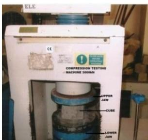
**Figure11:** Automatic Compression Testing Machine 3000KN
