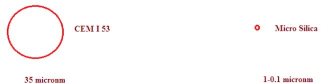
**Figure 3:** Particle size of cement and silica fume
