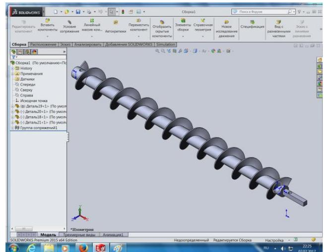
Figure 3. 3D model of the drilling auger
