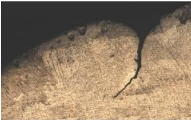
**Figure 2.** The microstructure of austenitic steel with a crack
