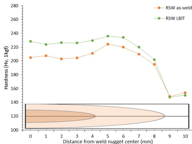
**Figure 7:** Microhardness profile for RSW LBIT and RSW as-weld samples using Hardness Vickers
