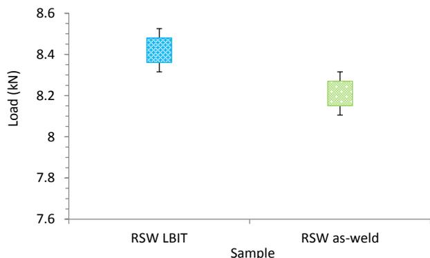
**Figure 5:** Tensile-shear Load of RSW LBIT and as-welded samples
