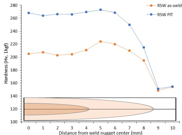
**Figure 6:** Microhardness profile for RSW PIT and RSW as-weld samples using Hardness Vickers
