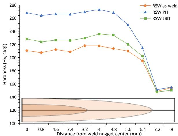
**Figure 8:** Microhardness profile for RSW PIT, RSW LBIT and RSW as-weld samples using Hardness Vickers
