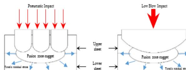
**Figure 1:** Schematic illustration on post-weld impact treatment process, (a) pneumatic impact treatment and (b) low blow impact treatment.
