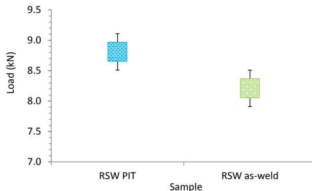
**Figure 4:** Tensile-shear Load of RSW PIT and as-welded samples
