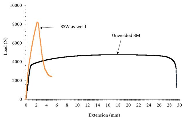
**Figure 3:** Tensile-shear curves.
