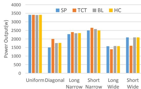
Figure 4: Comparison of power output under different shadings.
