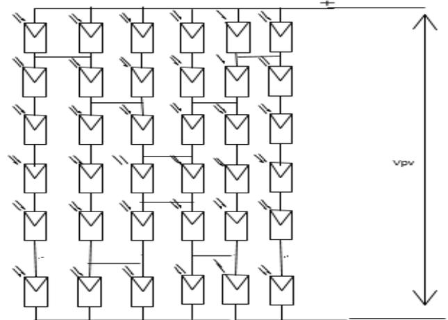
**Figure 1(c):** Solar modules connected in Honey comb (HC)
