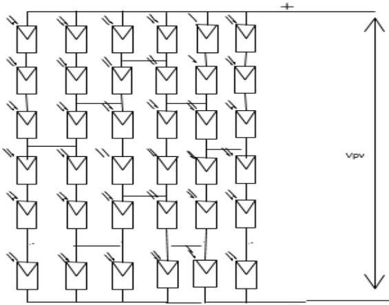
Figure 1(d): Solar module connected in Bridge Link (BL)
