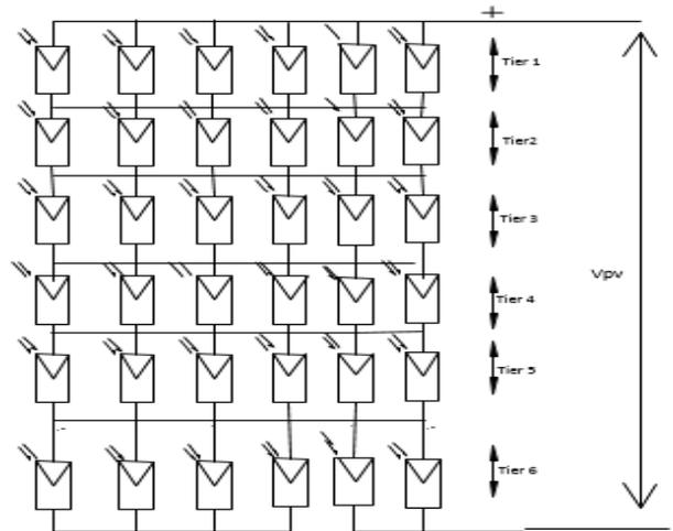
**Figure 1(b):** Solar modules connected in Total Cross Tied (TCT)
