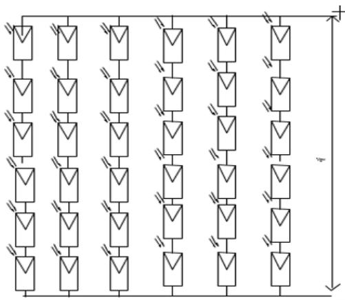
**Figure 1(a):** Solar modules connected in Series-Parallel (SP)
