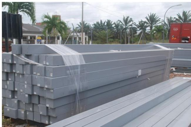
**Figure 1:** Example of Fiberglass crossarm
