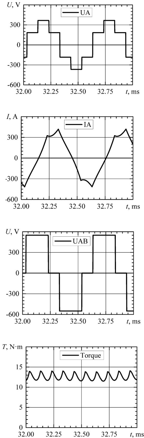
**Figure 2:** Results of mathematical modeling of electromagnetic processes in a high-speed generator: UA – phase voltage; UAB – line-to-line voltage; IA – phase current; Torque – electromagnetic torque
