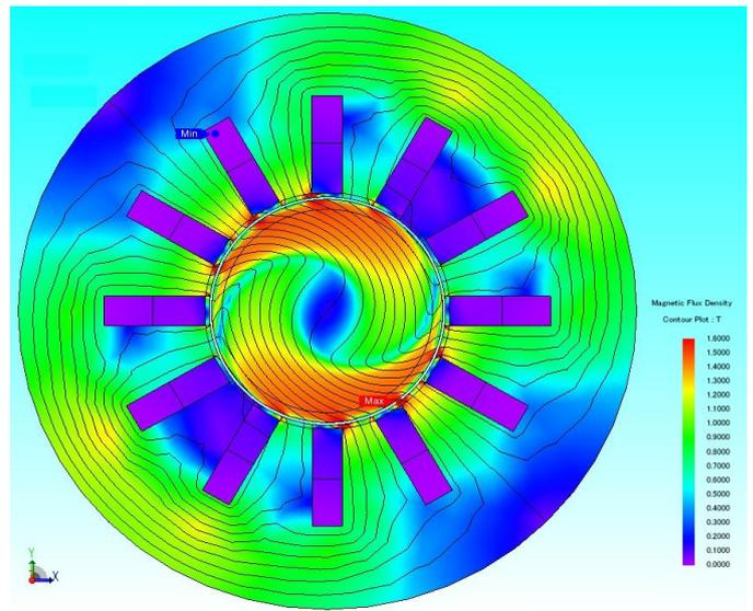
**Figure 3:** Distribution of magnetic field induction in the computational domain for a three-phase stator winding
