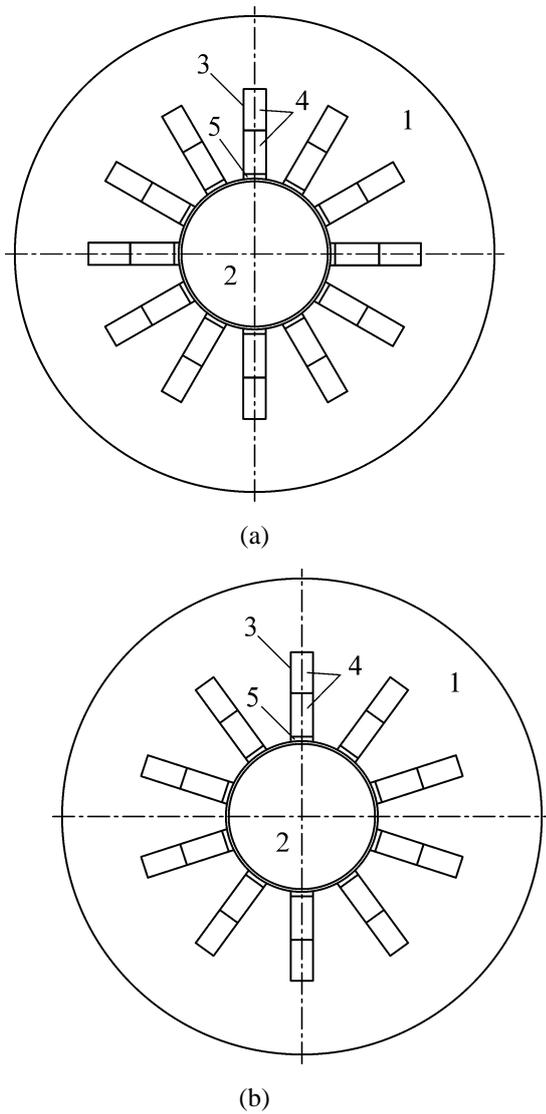
**Figure 1:** Sketches of high-speed electric generator active part for gas microturbine installations: (a) three-phase winding; (b) five-phase winding
