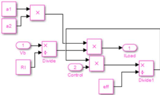
Figure 4: Simulink model of inverter and the load
