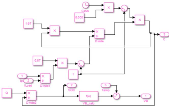
Figure 2: Simulink model of battery
