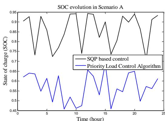
**Figure 7:** Evaluation of battery SoC for constant load profile
