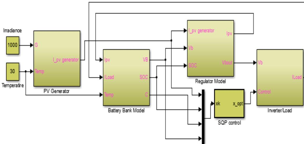
Figure 5: Simulink diagram for the stand alone PV system
