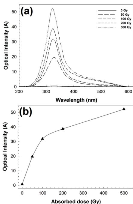
**Figure 3:** Absorption spectra of RPLGD with 3.5 mol% of silver activator concentrations irradiated with the different doses by Co-60 source. The irradiated dosages of glass were from 50 to 500 Gy with 0 Gy as a control.
