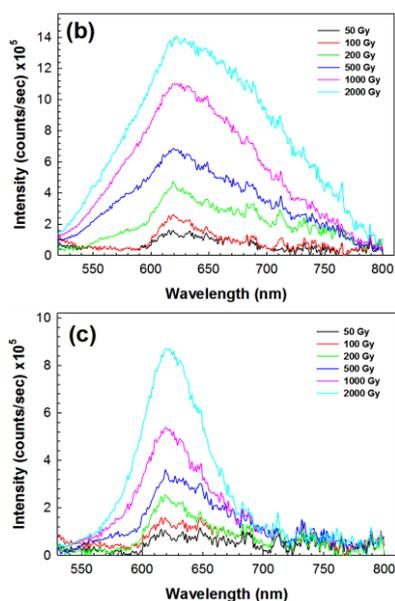
**Figure 5:** Emission spectrum of RPLGD samples (a) 2.0wt.%, (b) 4.0wt.% and (c) 8.0wt.% of silver contents at different irradiation doses. The samples were excited at 325 nm.
