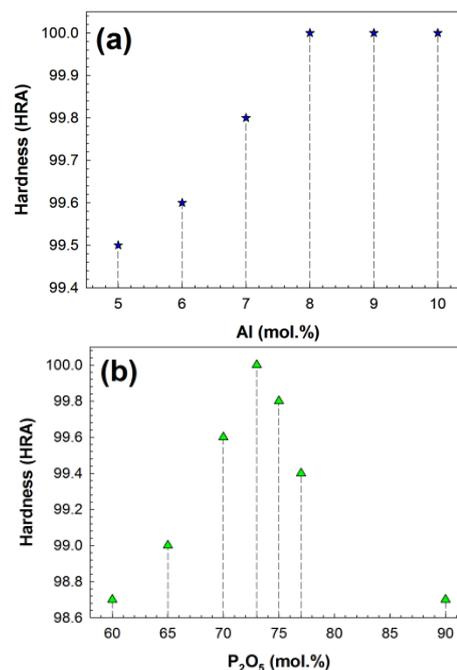
**Figure 4:** Distribution of Rockwell hardness of RPLGD with different wt.% of aluminium and phosphorus pentoxide contents
