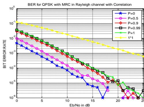
Figure 7: BER of QPSK in MRC in Rayleigh channel with Correlation
