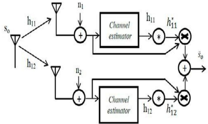
Figure 1: Maximal ratio combiner in digital communication system
