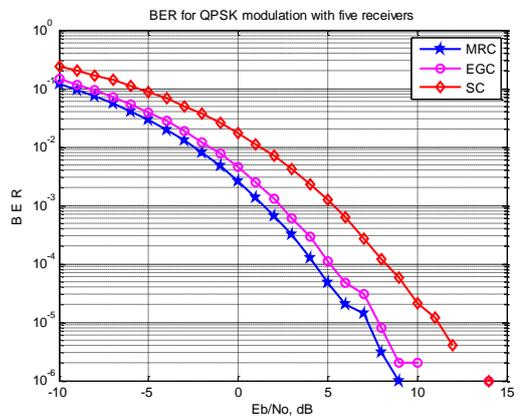
**Figure 6:** BER of BPSK in MRC ,EGC and SC using five receiver
