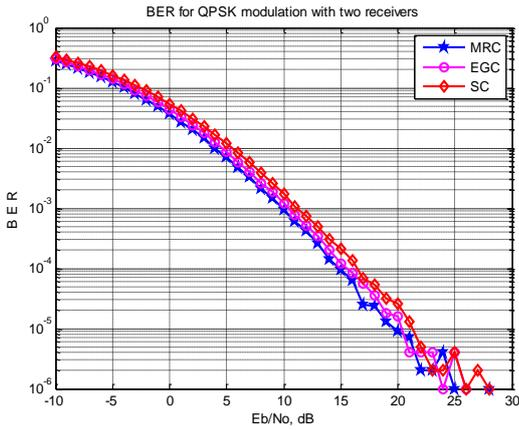
**Figure 2:** BER of BPSK in MRC,EGC and SC using two receiver
