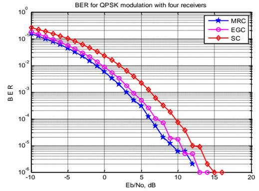
**Figure 5:** BER of BPSK in MRC ,EGC and SC using four receiver
