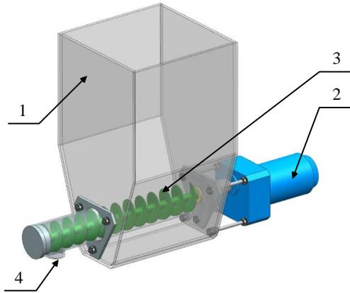
1 - bunker; 2 - motor without collector with reducer (type FL86BLS98); 3 - screw; 4 - feed box.
