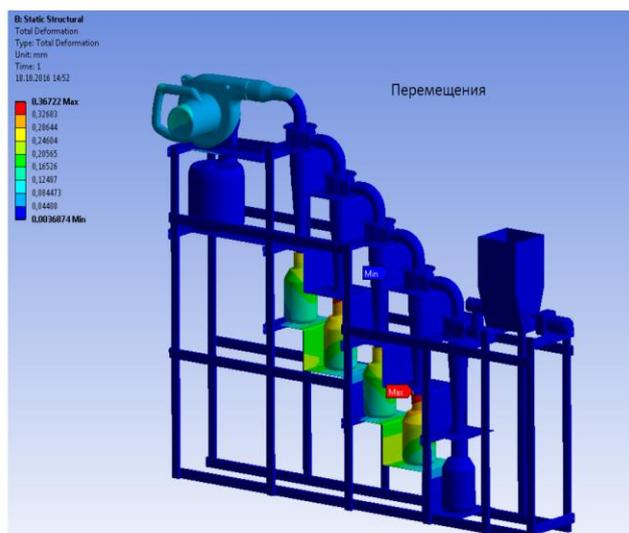
**Figure 5:** Curve of deformations in the stand design, mm (max 0,36mm.)
