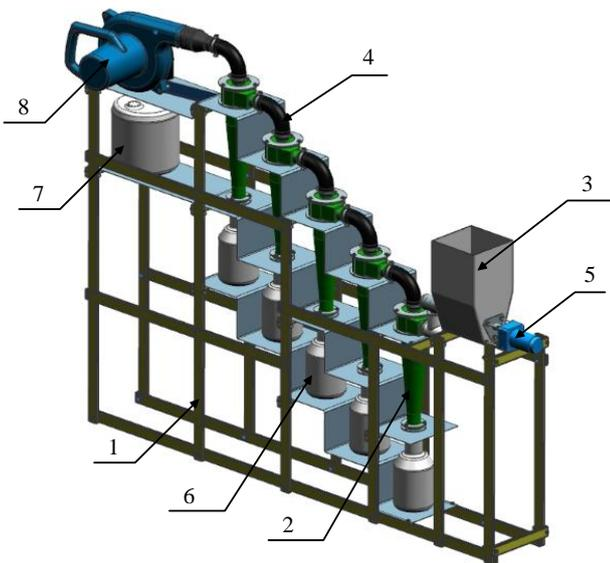
1 - frame; 2 - coagulant; 3 – loading hopper; 4 - flexible outlet; 5 – motor without collector with reducer (type FL86BLS98); 6 - container; 7 - container for collecting dust after blower; 8 - the electric blower (such as Makita UB1101).
