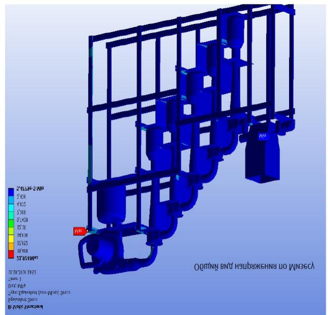
**Figure 4:** Curve of stresses on the Von-Mises in stand design, MPa (21.924 MPa max.)
