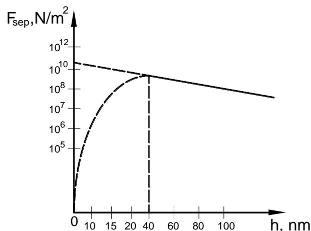
**Figure 2:** The dependence of adhesion  $F_{sep}$  from the film thickness  $h$
