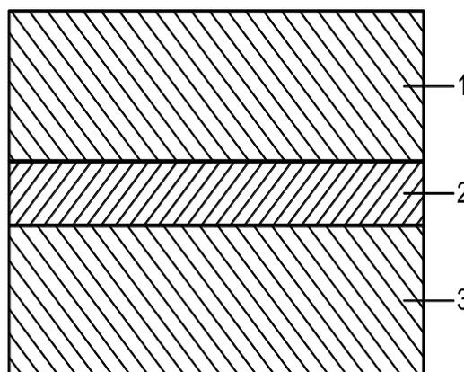
**Figure 1 a:** Structure in which two films are connected through a weakly-ferromagnetic layer (non-magnetic layer);
