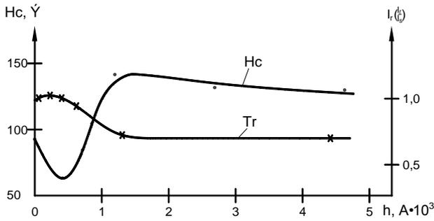
**Figure 3:** The dependence of the coercive force  $H_c$  and relative remanent magnetic induction  $j\left(\frac{I_r}{I_s}\right)$  from films thickness  $Co - Cr$ . The density of  $Cr$  is 10%
