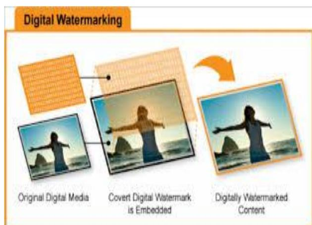
**Figure 3:** The conversion process from original media to digital watermarked content.
