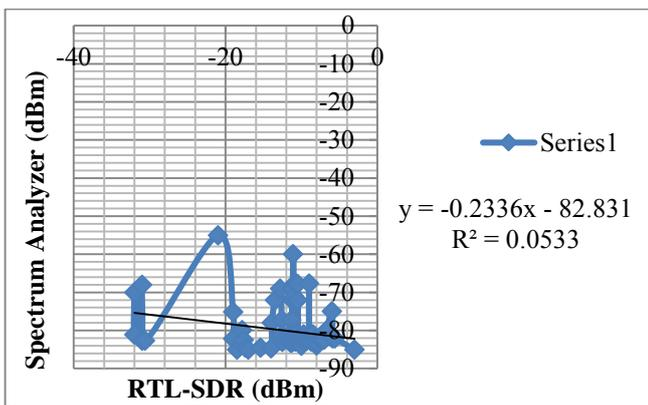
**Figure 4:** Linear regression between measurements using a spectrum analyzer and using android base RTL-SDR
