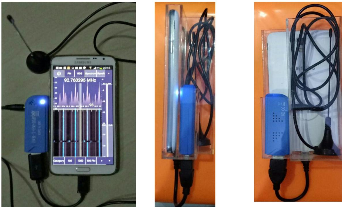
**Figure 3:** Android spectrum analyzer with RTL-SDR (a) Front view, (b) Side view, (c) Back view
