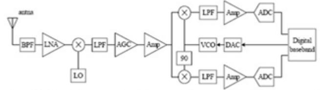
**Figure 1:** Block diagram of Analog Transceiver
