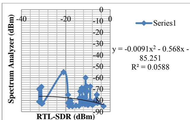
**Figure 5:** Second order regression between measurements using a spectrum analyzer and using android base RTL-SDR
