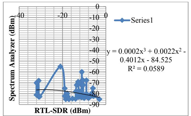
**Figure 6:** Third-order regression between measurements using a spectrum analyzer and using android base RTL-SDR
