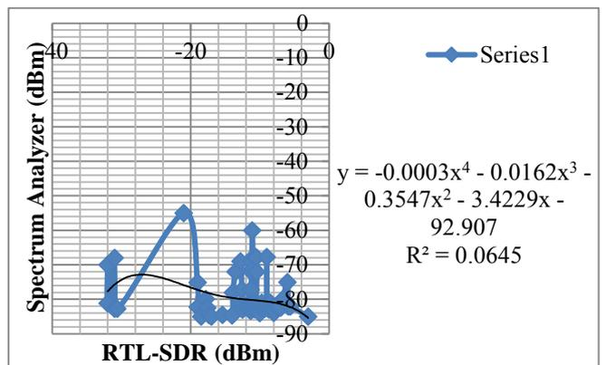
**Gambar 7:** Fourth-order regression between measurements using a spectrum analyzer and using android base RTL-SDR
