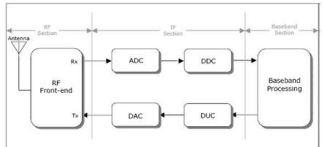
**Figure 2:** SDR Transceiver
