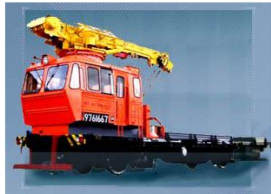
**Figure 2:** The loading transport locomotive LTL-6 (overview)
