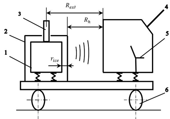
**Figure 7:** The calculation scheme for the formation of noise spectra of the air component in the cabin:
