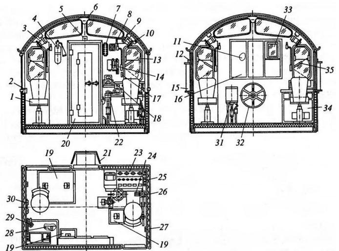
**Figure 5:** The location of the equipment in the cab (foot-plate) of the locomotive driver SML2:
