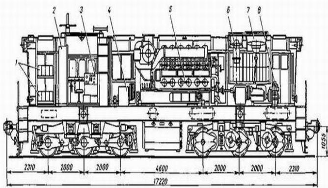
**Figure 6:** The location of the equipment on the locomotive of the ChME3 series:
