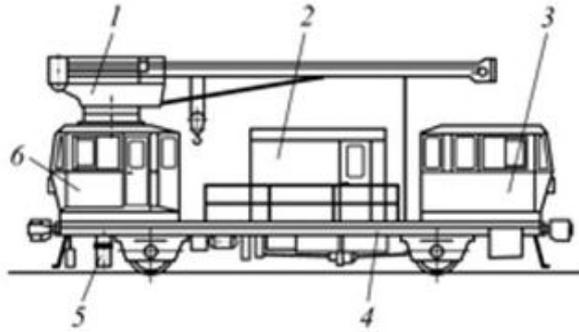
**Figure 3:** The configuration of the loading transport locomotive LTL-6 (overview): 1 - the jib of the crane; 2 – the locksmith's workshop; 3 – the cabin for transportation of mechanized brigades; 4 – the platform of the locomotive; 5 - outriggers; 6 – the control foot-plate
