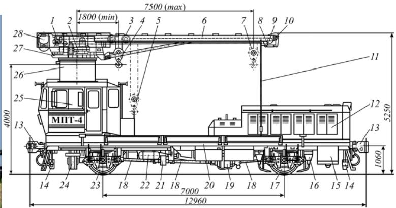
**Figure 1:** The configuration of the loading transport locomotive LTL-4 (overview):
