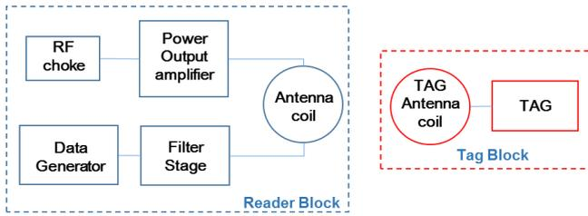
Figure 1: RFID System basic architecture.
