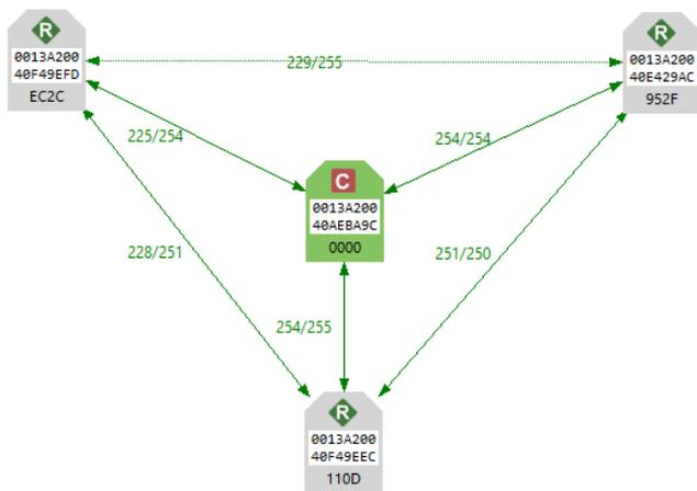
Figure 2: Zigbee wireless network in Mesh topology.
