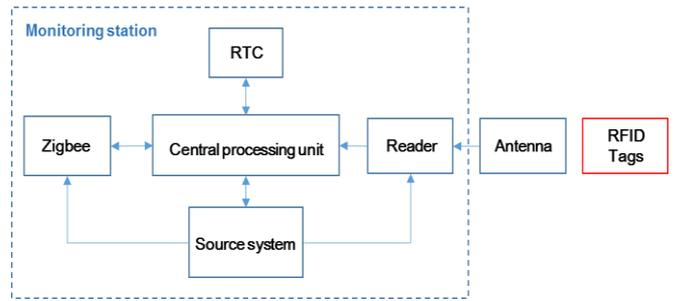
Figure 3: Block diagram of the proposed system.
