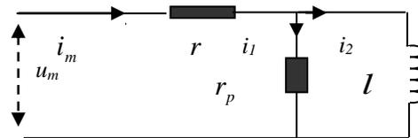
**Figure 1:** The iron core coil
