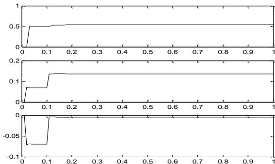
**Figure 4:** Identification of numerical parameters versus time (s)  $a_1$  (top);  $b_1$  (middle), and  $c_1$  (bottom)
