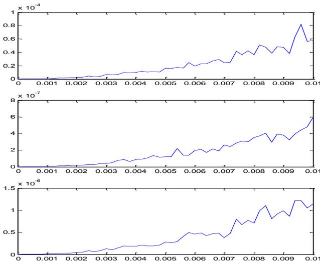
**Figure 8 :** Variance numerical parameters estimated in accordance with the magnitude of the measurement error;  $a_1$  (top);  $b_1$  (middle);  $c_1$  (low)
