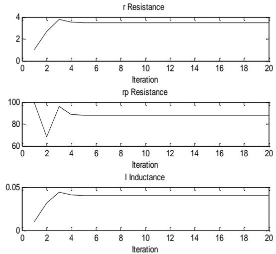
**Figure 6:** Identification of physical parameters in the number of iteration;  $r$  (above);  $r_p$  (middle);  $l$  (bottom)
