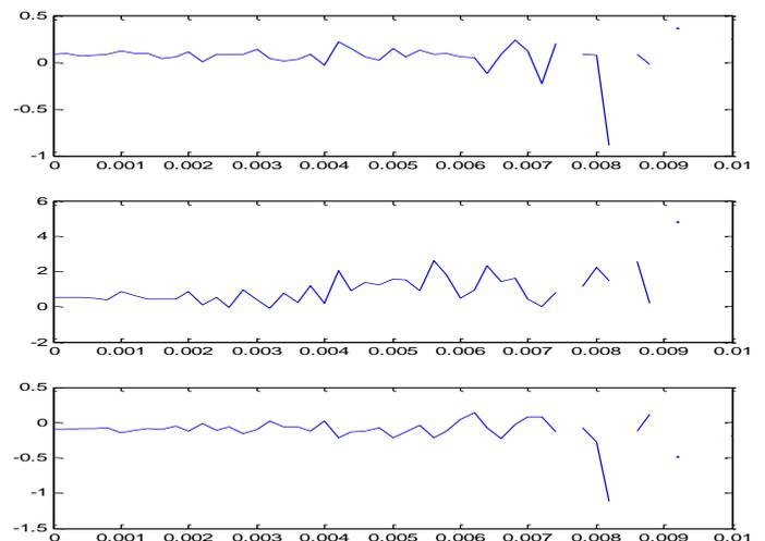
**Figure 10 :** Mean error estimation for the physical parameters depending on the magnitude of the measurement error;  $r$  (above);  $r_p$  (middle);  $l$  (bottom)
