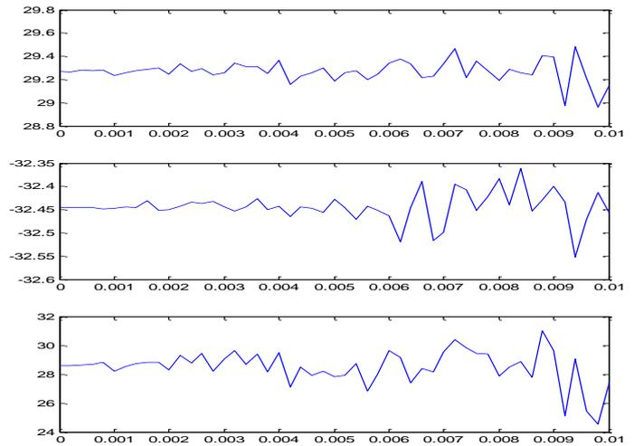
**Figure 9 :** Estimated average error of digital parameters in accordance with the magnitude of the measurement error;  $a_1$  (top);  $b_1$  (middle);  $c_1$  (low)
