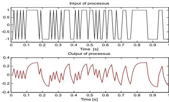
**Figure 3:** Sequence input-output versus time (s), sequence pseudo-random binary input (top), actual output (low, solid lines) and measured (bottom dotted lines)
