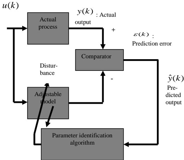
**Figure 2:** The principle of identification
