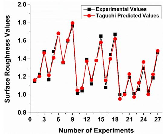
**Figure 6:** Relationship among the experimental and predicted results of surface roughness
