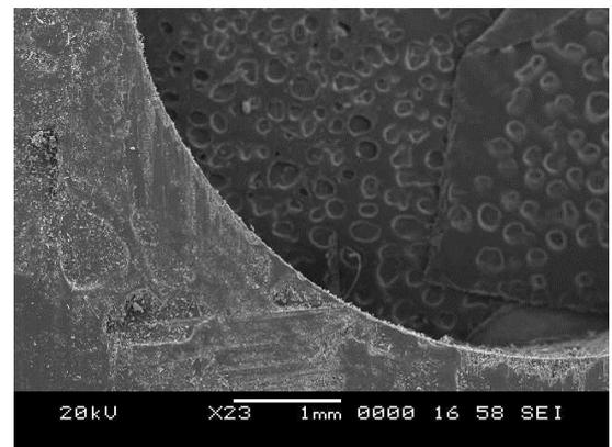
**Figure 9:** SEM image of the hole drilled for optimum cutting parameters
