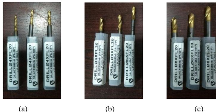
Figure 2: TiN coated carbide drills (a) 4 mm (b) 6 mm and (c) 8 mm.
