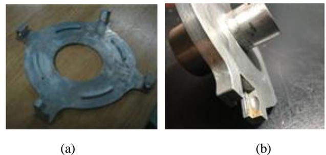
**Figure 1:** Damage of Oldham ring and the orbiting scroll wrap [3].
