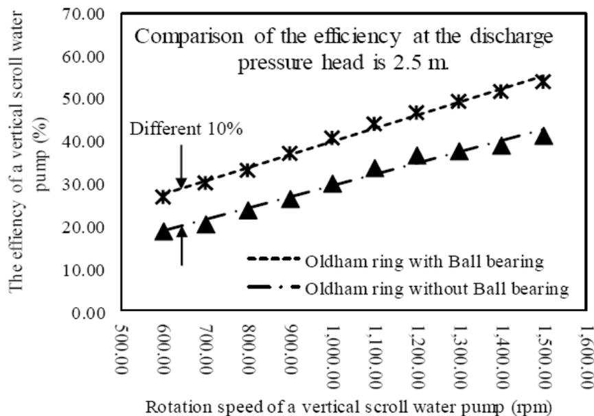
**Figure 8:** Comparison of the efficiency of a vertical scroll water pump at the discharge pressure head is 2.5 m.
