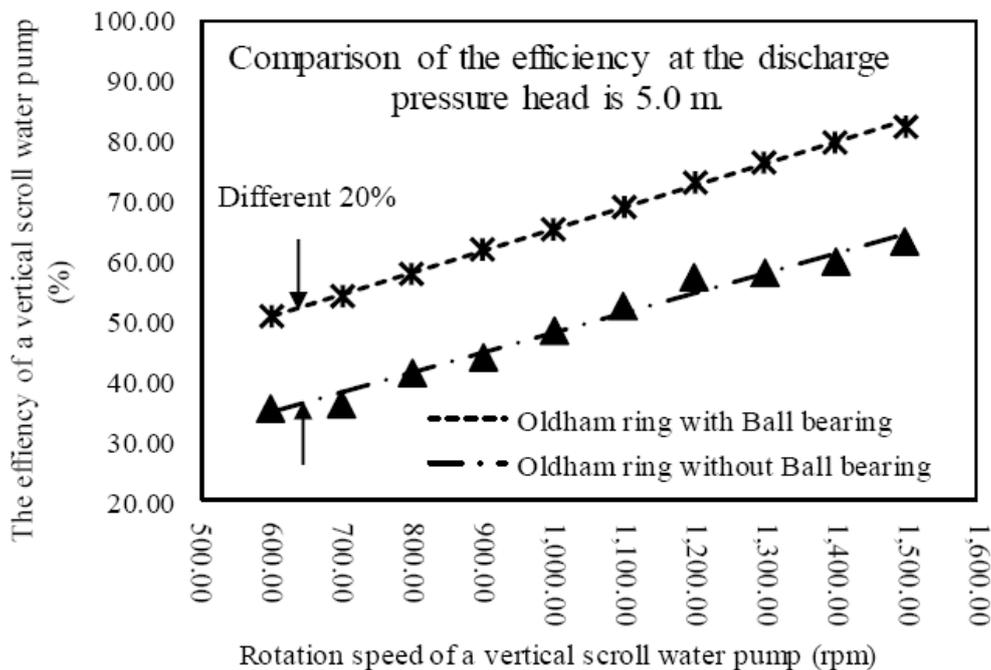
**Figure 10:** Comparison of the efficiency of a vertical scroll water pump at the discharge pressure head is 5.0 m.
