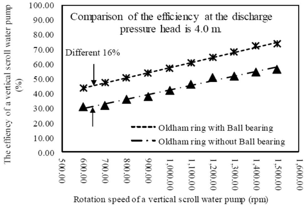
**Figure 9:** Comparison of the efficiency of a vertical scroll water pump at the discharge pressure head is 4.0 m.
