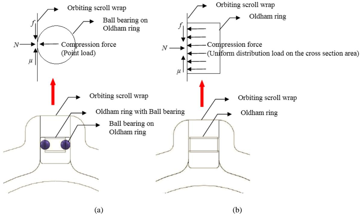
**Figure 2:** Compression force between Oldham Ring and Orbiting scroll wrap.
