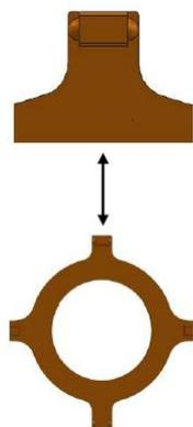
**Figure 3:** Oldham ring with Ball bearing
