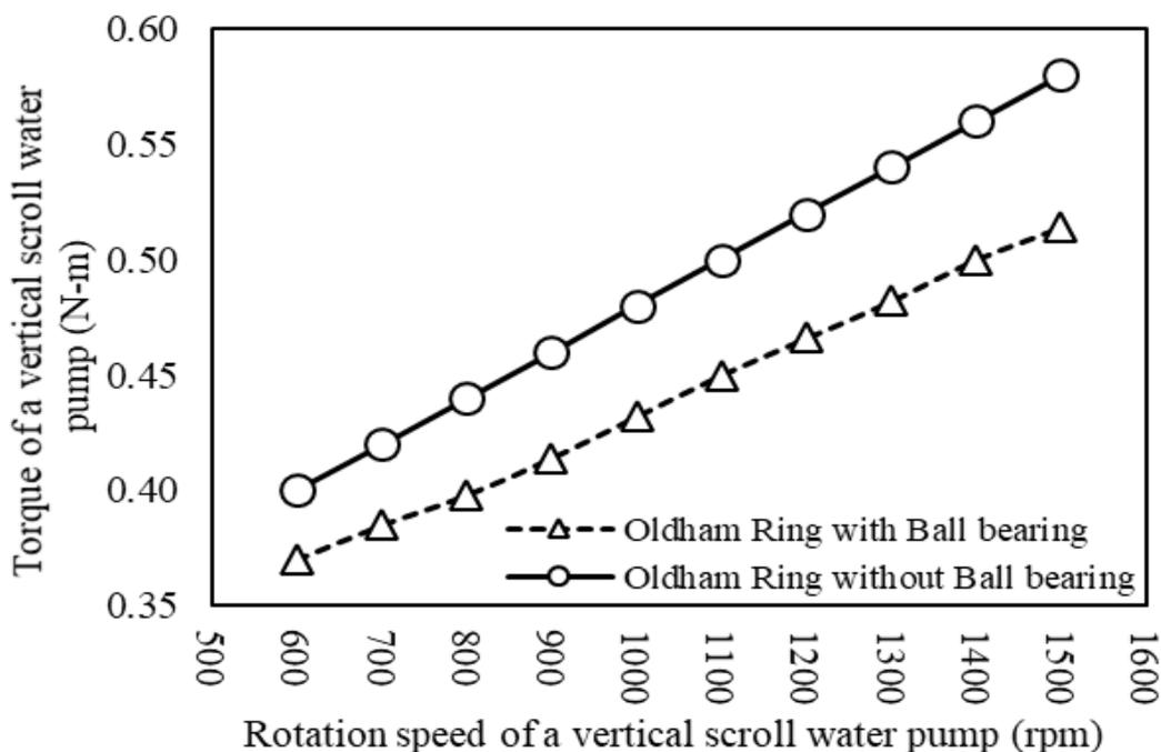
**Figure 5:** Comparison of the torque of a vertical scroll water pump used the Oldham ring
