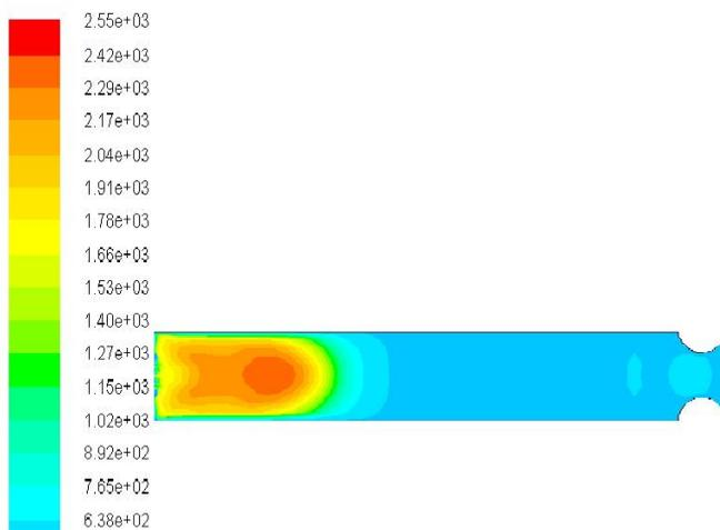
Fig. 16 combustion progress near the injector
