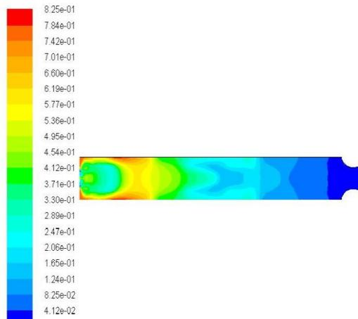
Fig 14 Contours of mole fraction of H<sub>2</sub>O
