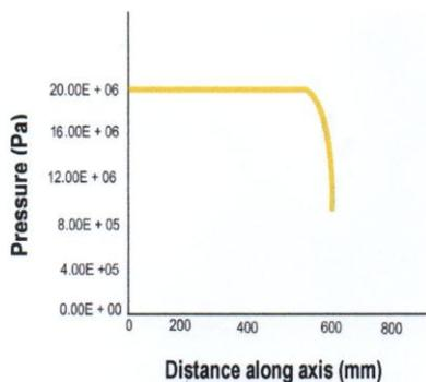
Variation of pressure along thrust chamber without cooling
