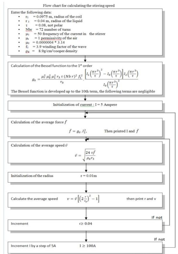
Figure 13: Chart for calculating of stirring speed
