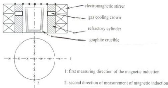
**Figure 8:** Measuring the magnetic induction in two directions.
