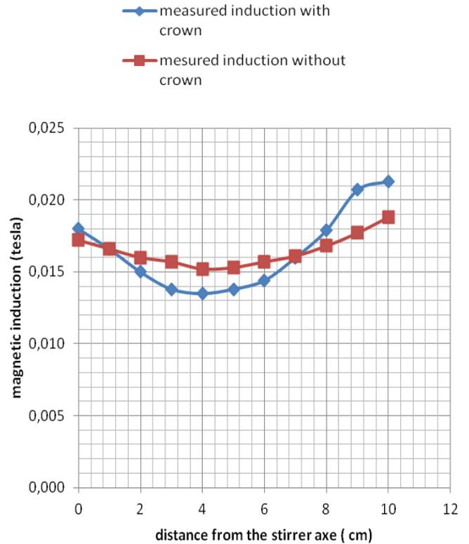
**Figure 9:** Variation of the magnetic induction (B) as function of the diameter of the stirrer
