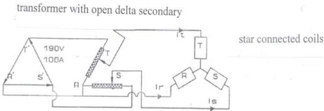
**Figure 6:** Supply circuit of the stirrer coils R- S- T
