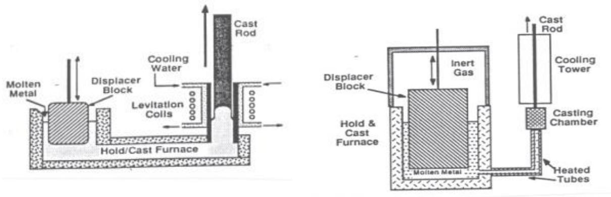
Figure 1: component of the levitation casting process
