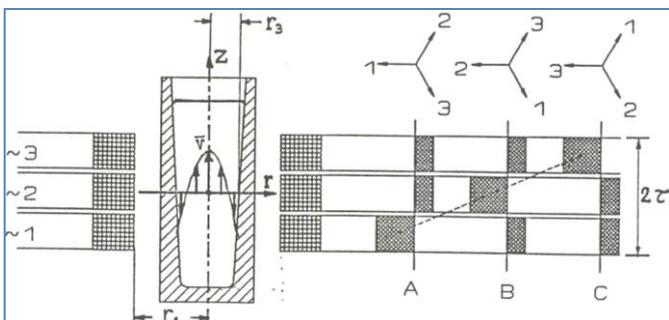
**Figure 12:** Three-phase winding of a cylindrical stirrer
