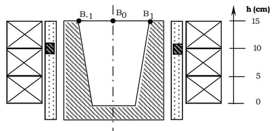
**Figure 10:** Marking the measuring points of the stirrer induction
