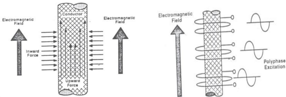
Figure 2: Component of the levitation casting process model. Hugh R;Lowry [3]
