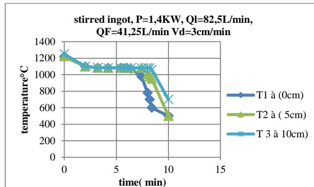
Figure 15: Temperature variation in the case with stirring.
