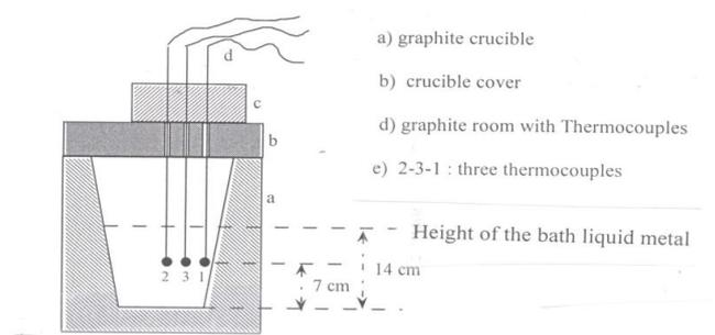
**Figure 19:** device used to measure the temperature along the diameter
