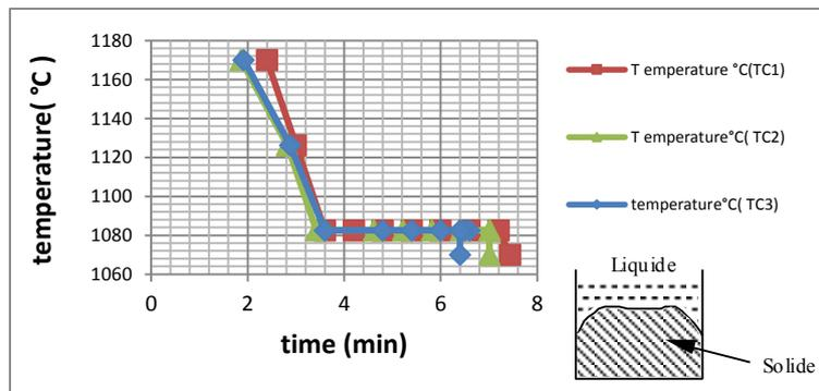
**Figure 20:** temperature measurement of the diameter of the ingot with stirring
