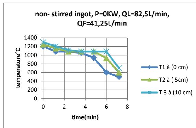
Figure 16: Temperature variation in the case without stirring.
