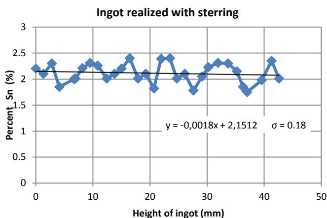
**Figure 18:** Variation of tin proportion following the height of the ingot
