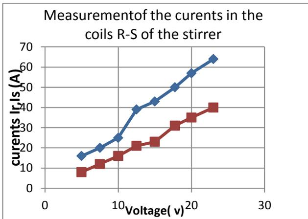
**Figure 7:** Measurement of the  $I_r$  and  $I_s$  currents in the R-S coil of the stirrer as a function of the voltage.
