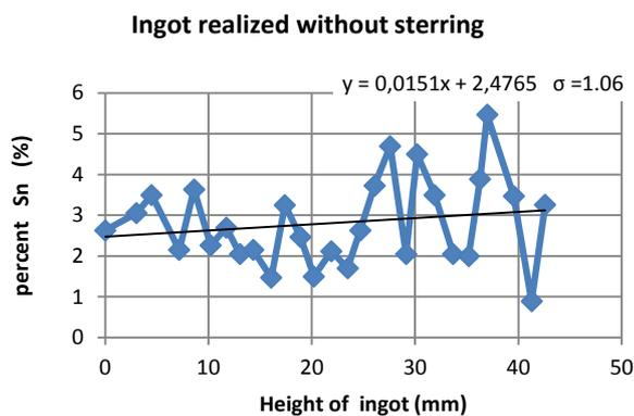
**Figure 17:** Variation of tin proportion following the height of the ingot
