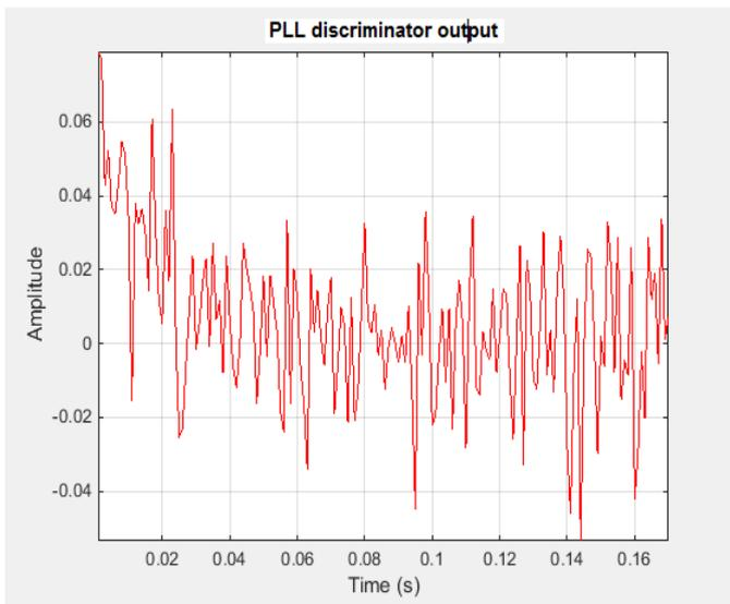
**Figure 4:** Phase error plot of carrier tracking loop
