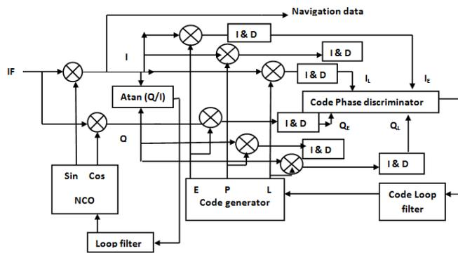
Figure 1: Combined carrier and CA code tracking loop
