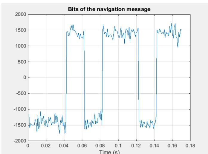
**Figure 6:** Extracted Navigation binary data
