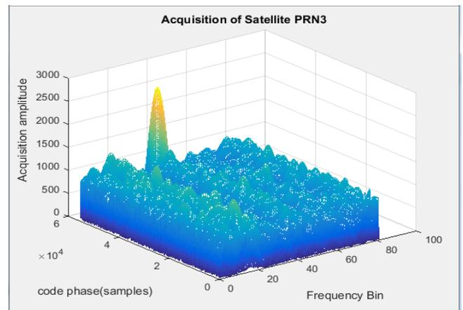
Figure 2: Correlation peak power of PRN3 satellite signal
