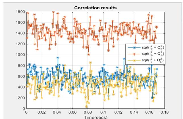
Figure 3: Correlation power plot of I and Q channel
