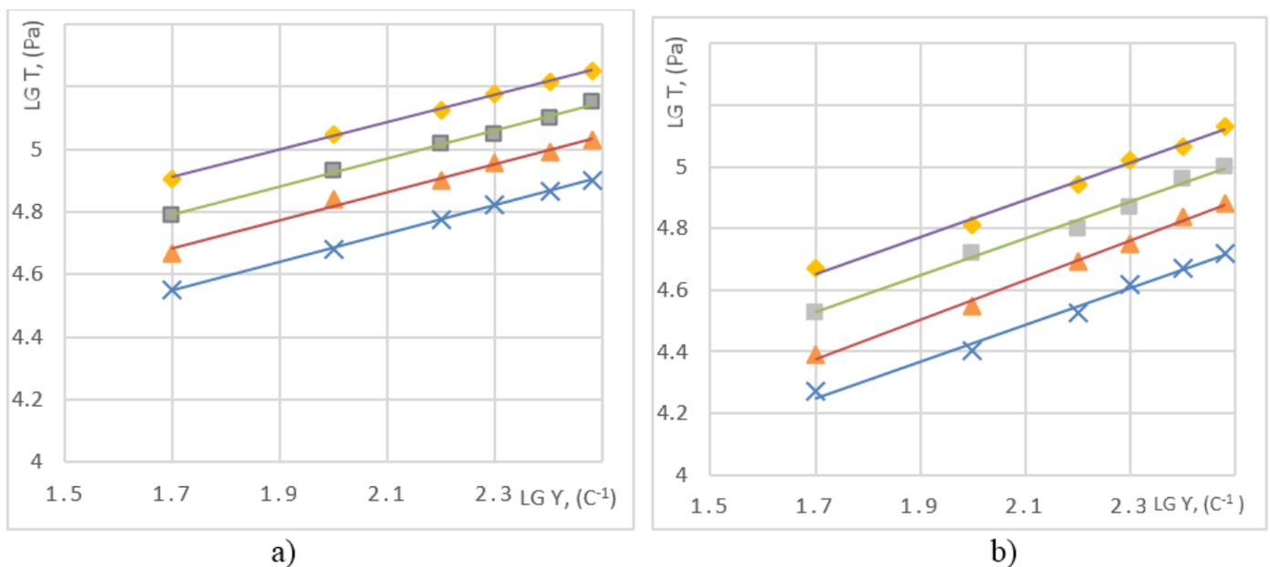
**Figure 1:** Flow curves of pro-oxidant additive, containing 5.0 % by mass of cobalt stearate, through capillaries with a diameter  $d = 1$  mm, lengths: a)  $l = 5$  mm and b)  $l = 30$  mm at a temperature of:
