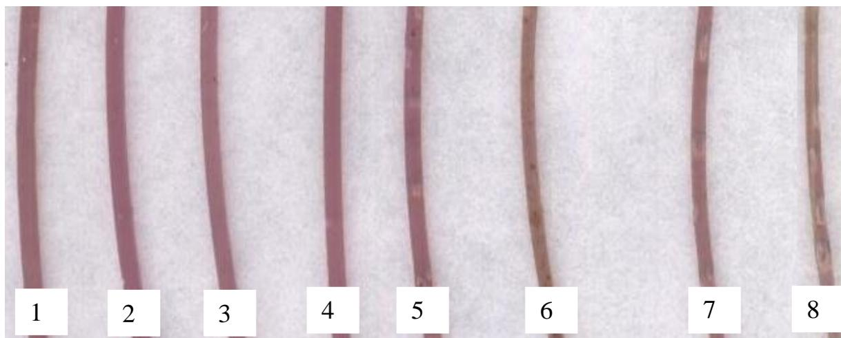
**Figure 2:** Photos of pro-oxidant additive extrudates containing 10% by mass of cobalt stearate when flowing through a capillary with a diameter  $d = 1$  mm and length  $l = 5$  mm in the temperature range, °C:
