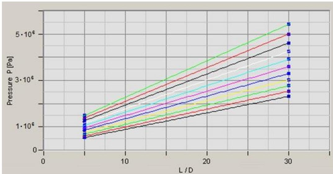
**Figure 5:** Pressure values before the forming tool extrapolated to the zero chamber length for PVD 15803-020 with a cobalt stearate content of 10% by mass.
