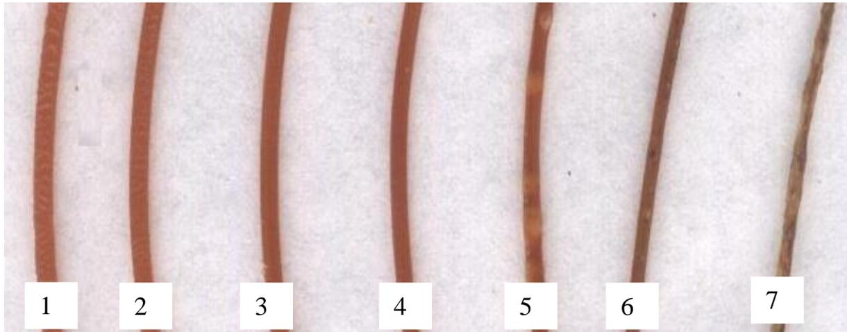
**Figure 3:** Photos of pro-oxidant additive extrudates containing 10% by mass of cobalt stearate when flowing through a capillary with a diameter  $d = 1$  mm and length  $l = 30$  mm in the temperature range, °C:
