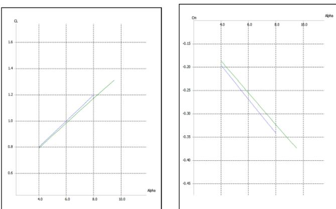
**Figure 5:**  $C_{L_{max}}$  vs  $\alpha$  and  $C_m$  vs  $\alpha$  for GA(green) and TLBO(blue)
