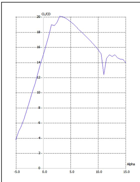
**Figure 2:**  $C_L/C_D$  variation with  $\alpha$
