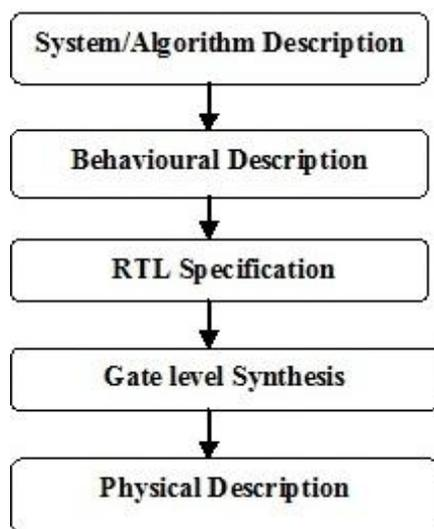
**Figure 1:** Design flow for FPGA based single chip solution
