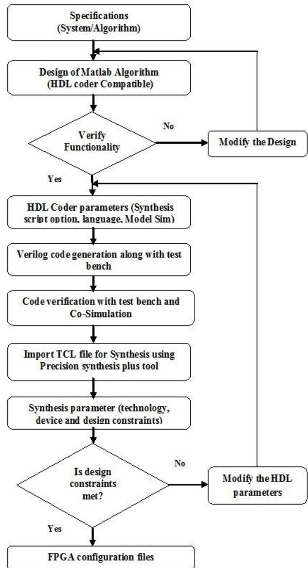
Figure 3: Flow chart depicting the design flow performed
