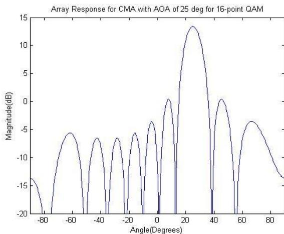
**Figure 5:** Array response gain using NCMA
