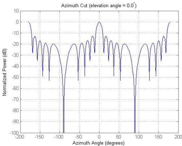
**Figure 4:** Array response before beamforming
