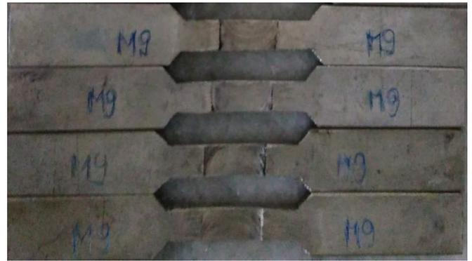
**Figure 2:** Tensile Samples of AE42 alloy
