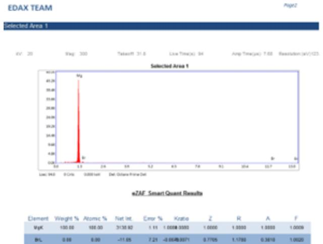
**Figure 11:** SEMEDX spectrum of Mg alloy AE42 base metal.
