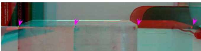
Figure 8: Four Pixels Identified on the Concatenated Rectified Stereo Images to be used for the Distance Measurement
