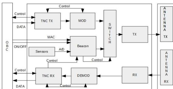
**Figure 3.** Critical Design of the communication module<sup>13</sup>
