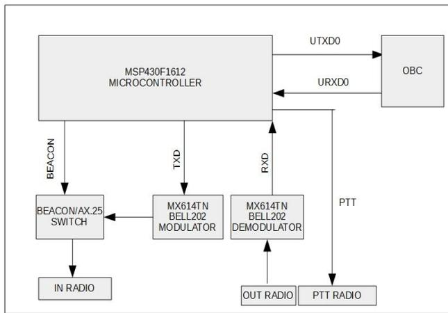
Figure 13: Block Diagram of the Communication Module<sup>27</sup>.
