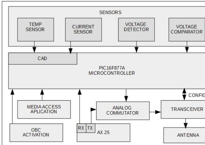
**Figure 6:** Hardware block System from the communication module<sup>13</sup>.
