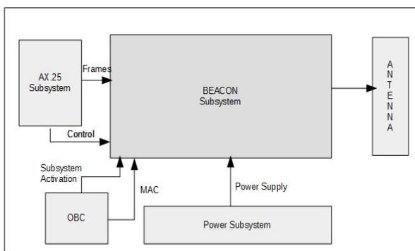
**Figure 5:** Inputs and Outputs of the submodule Beacon with another picosatellite modules<sup>13</sup>
