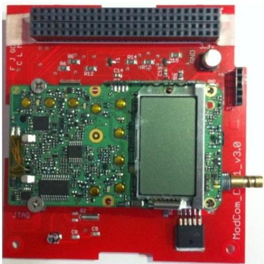
Figure 14: Final Version with YAESU VX 3 transceiver attached<sup>27</sup>.
