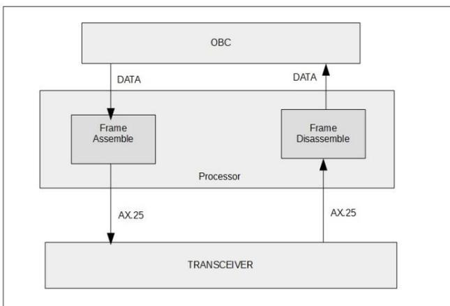
Figure 12: Block Diagram of the AX.25 Protocol<sup>23</sup>
