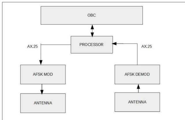
Figure 11: Block Diagram of the Transceiver Submodule<sup>23</sup>.
