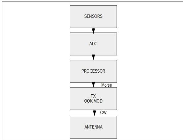
Figure 10: Block Diagram of the Beacon Submodule<sup>23</sup>.
