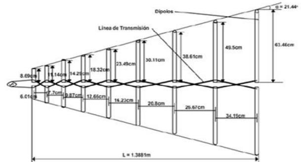
Figure 2: Design of the log-periodic antenna<sup>11</sup>
