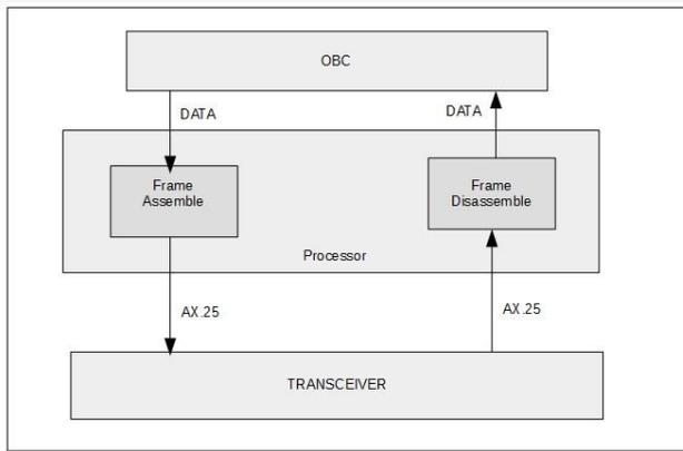
**Figure 7:** Block Diagram of the AX.25 Protocol<sup>23</sup>
