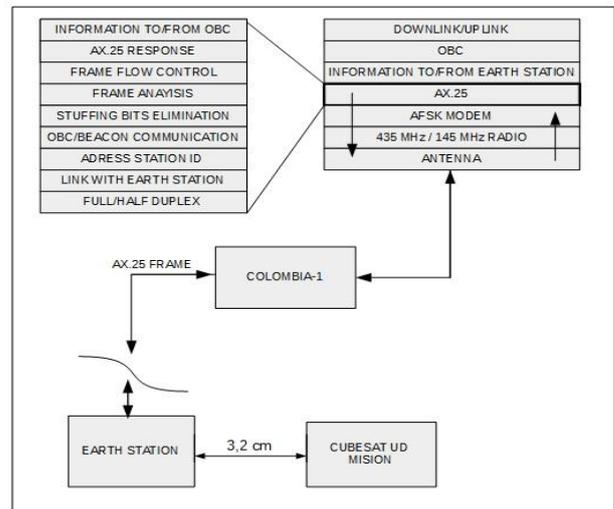
Figure 9: Blocks Diagram of AX.25<sup>22</sup>.
