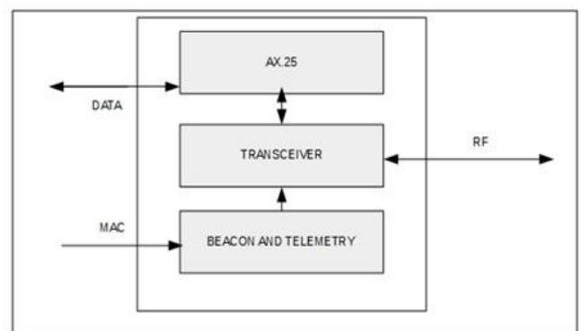
**Figure 1:** Block System of the Communication Module Colombia 1.<sup>8</sup>
