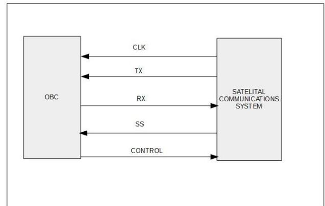
**Figure 8:** Lines between the communication module and OBC<sup>23</sup>.
