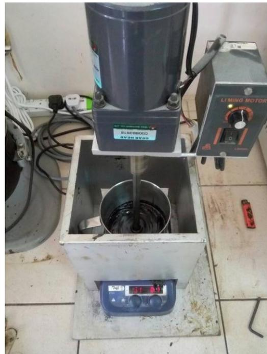
**Figure 1:** Mechanical mixer used to blend NRL with bitumen
