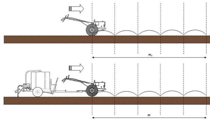
**Figure 2:** Schematic of wheel slip measurement
