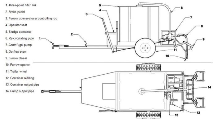
**Figure 1:** Schematic (side and top view) of biogas sludge applicator prototype
