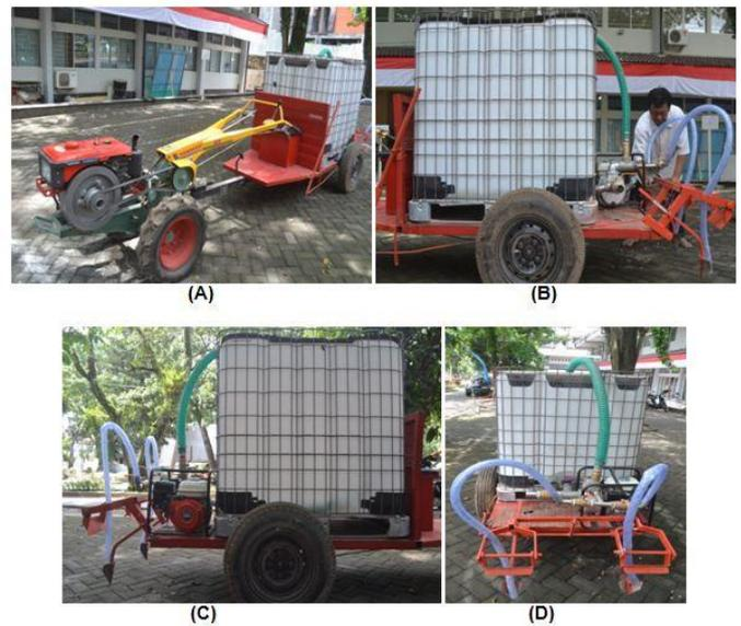
**Figure 3:** Biogas sludge applicator: (A) hand tractor as traction source, (B) sludge applicator and its sludge container, (C) sludge pump and piping system, (D) two furrow opener-closer at the back of applicator
