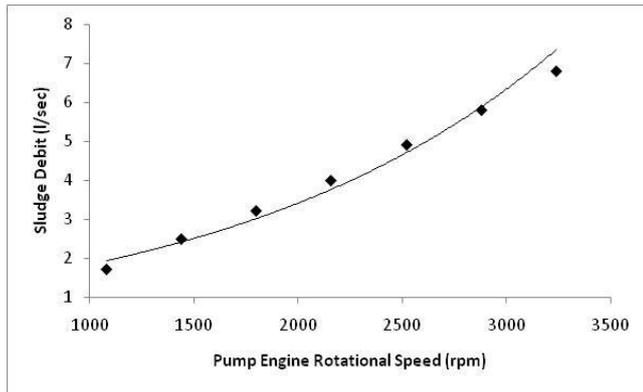
**Figure 4.** Biogas sludge debit at different pump engine rotational speed
