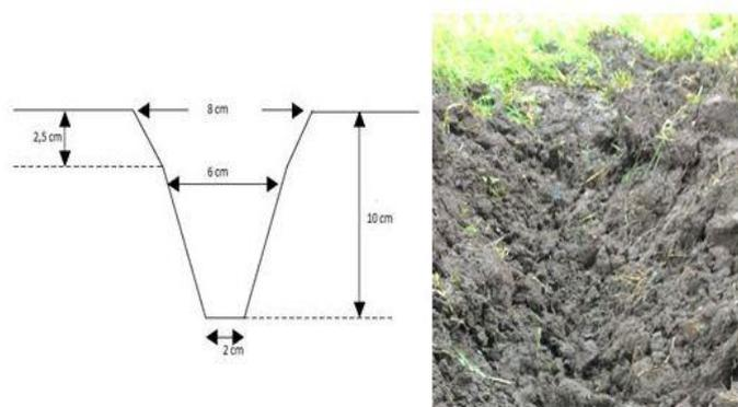
**Figure 5:** Cross-section profile of furrow made by furrow opener
