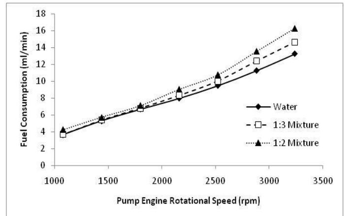
**Figure 6.** Fuel consumption (ml/min) at different pump engine rotational speed and different sludge mixture
