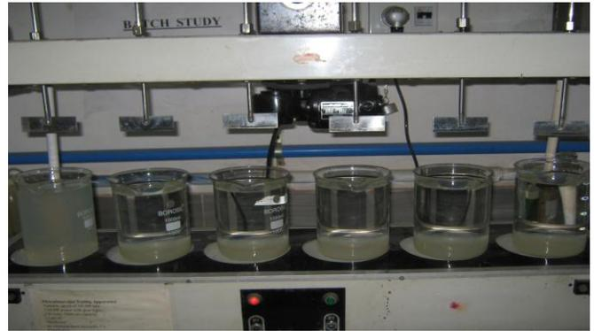
Photograph Showing the Removal of Turbidity at Different Dose of PAC Using Jar Test Apparatus.
