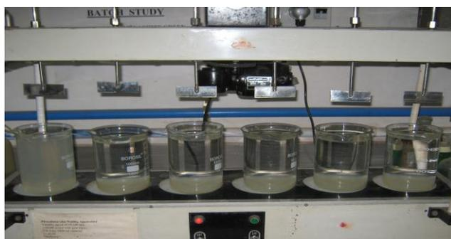
Photograph Showing the Removal of Turbidity at Different Dose level of Alum Using Jar Test Apparatus.
