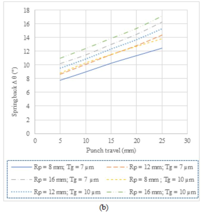
**Figure 2.** Effect of punch radius on spring back
