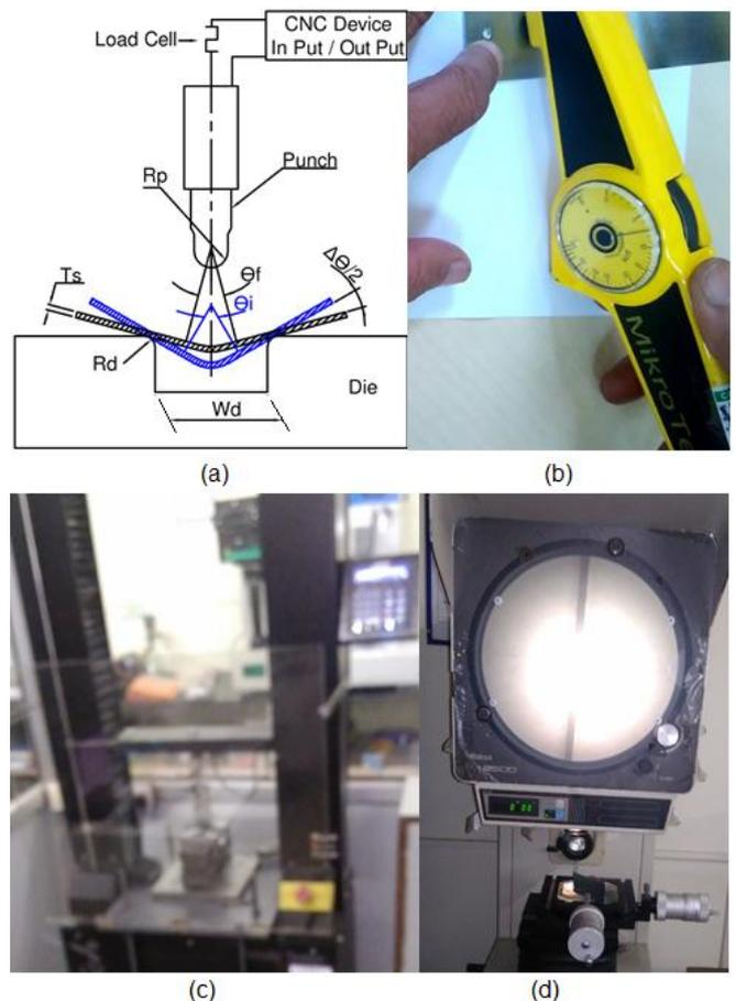
Figure 1. Experimental setup (a) schematic diagram of air bending and spring back (b) measuring the galvanizing thickness (c) bending setup on universal testing machine (d) profile projector for measurement of final bent angle.
