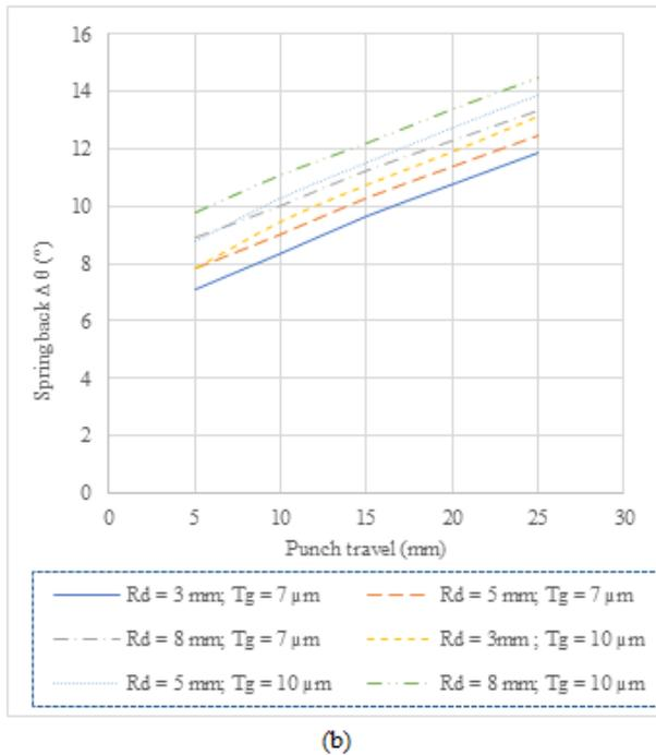
**Figure 3.** Effect of die radius on spring back
