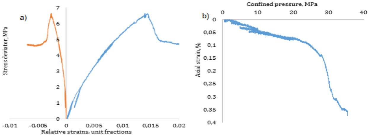
**Fig. 4.** Typical strain diagram of Proterozoic clay upon volumetric compression: a – triaxial compression; b – isotropic compression.
