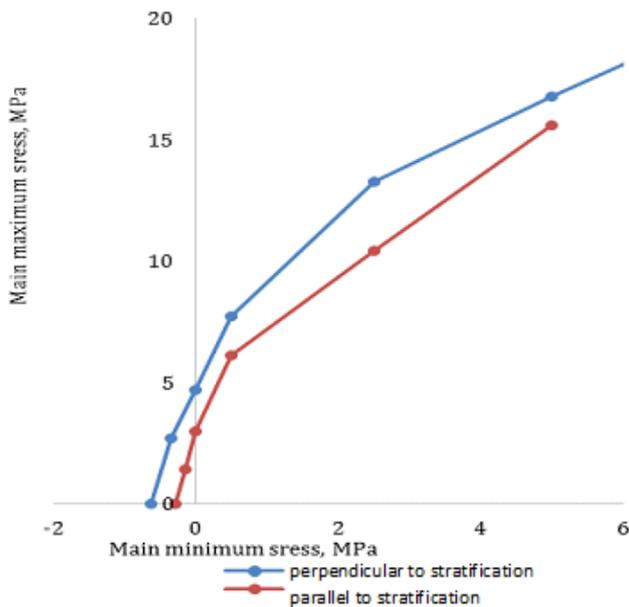
**Fig. 6.** Strength certificate of Proterozoic clay in the axes of main stresses (specimen taken from bottom of "Prospekt Slavy" Metro Station).
