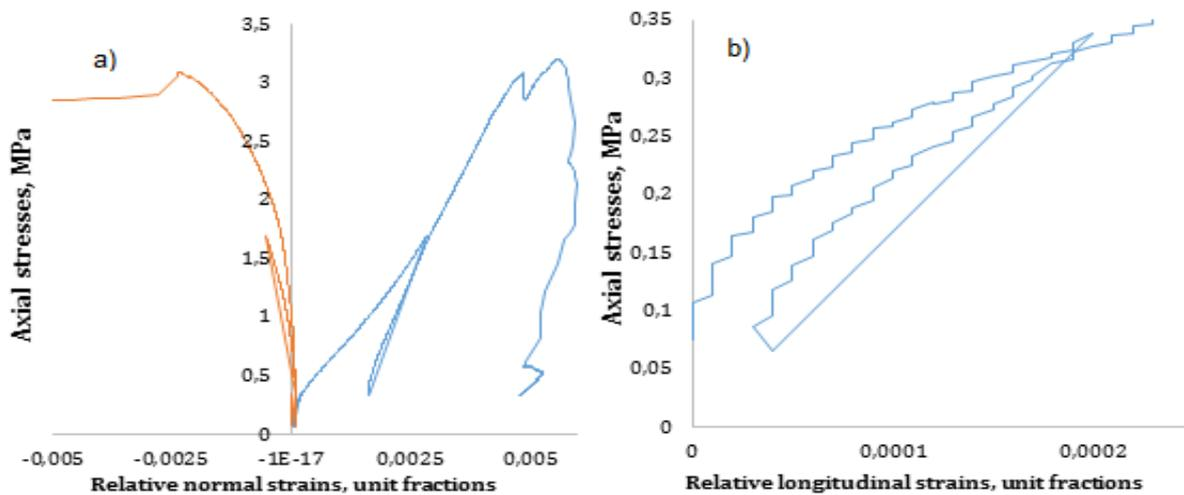
**Fig. 1.** Typical deformation pattern of Proterozoic clay: a – total deformation diagram; b – interaction between axial stresses and longitudinal strains in the range of minor strains
