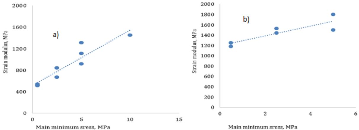
**Fig. 5.** Rock strain modulus as a function of confined compression ("Prospekt Slay" Metro Station: a – tests in perpendicular to stratification; b – in parallel to stratification).
