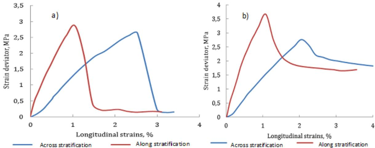
**Fig. 3.** Characteristic behavior of Proterozoic clay in parallel and perpendicular to stratification: a – lateral pressure  $\sigma_3 = 0$ ; b – lateral pressure  $\sigma_3 = 0.5$ .
