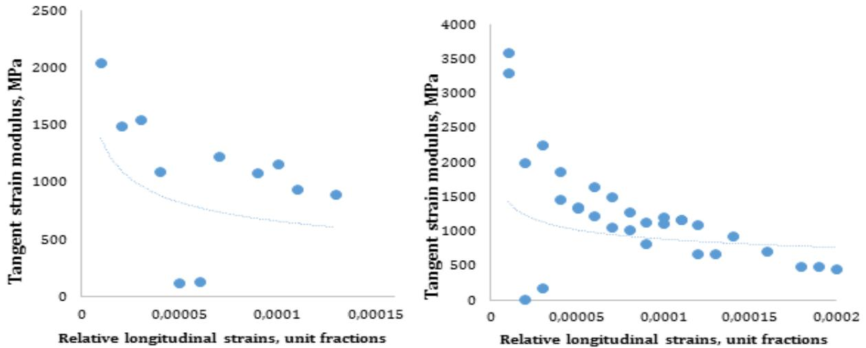
**Fig. 2.** Variation of tangent strain modulus of Proterozoic clay as a function of achieved value of relative longitudinal strains (typical dependences).
