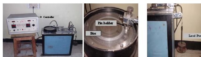
Figure 1: Pin-On-Disc Type Friction and Wear Monitor With Data Acquisition System
