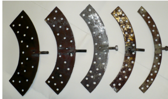
Figure 2. A set of changeable blades of the triple-threaded helix.
