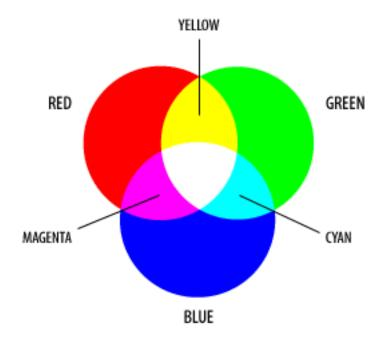
The added substance model of RGB Red, green, and blue are the essential boosts for human color observation and are the essential added substance colors.
