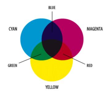
The colors created by the subtractive model of CMYK don't look exactly like the colors created in the additive model of RGB Most importantly, CMYK cannot reproduce the brightness of RGB colors. In addition, the CMYK gamut is much smaller than the RGB gamut.
