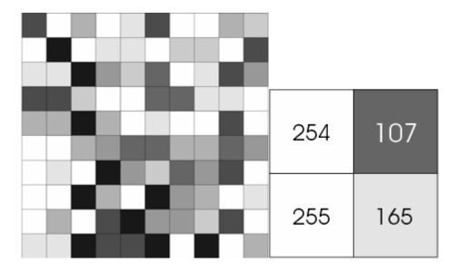
Each pixel has a value starting from 0 (black) to 255 (white). The possible range of the pixel values depend on the color depth of an image, here 8 bit is equal to 256 tones or grey scales.
