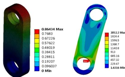
(a) Deformation (b) Bending Stress
