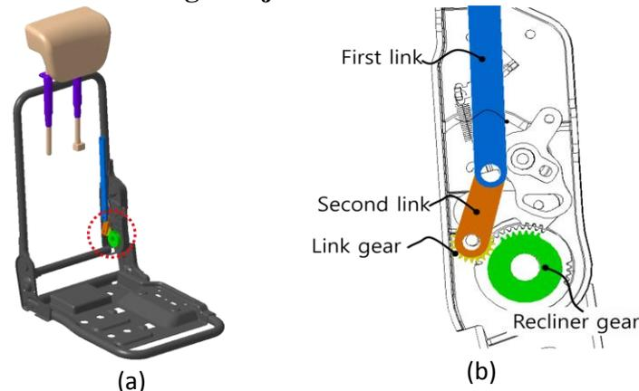
Fig. 3 Modeling of height adjustment mechanism
