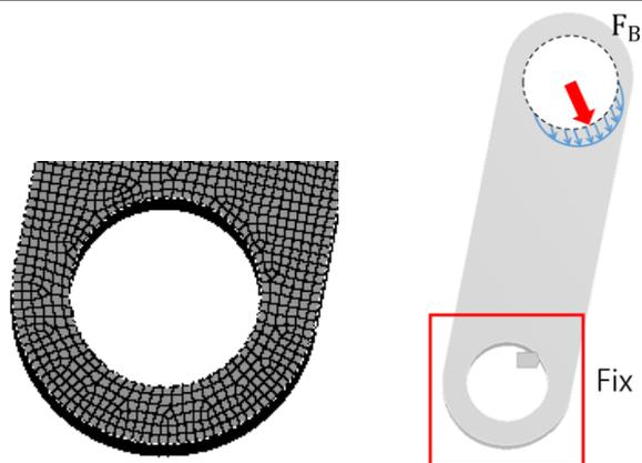
Fig. 8 Mesh and force condition
