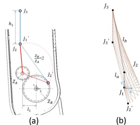
Fig. 4 Simulation of link motion in a recliner case
