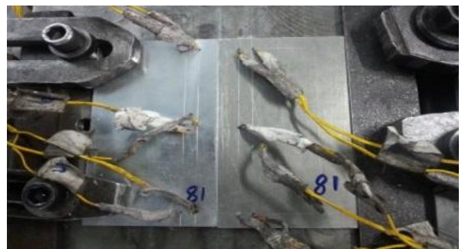
Fig. 4 Arrangement of thermocouples before welding
