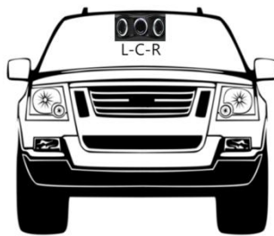
Fig. 4. Test model for blackbox installed vehicle with 3 camera lenses
