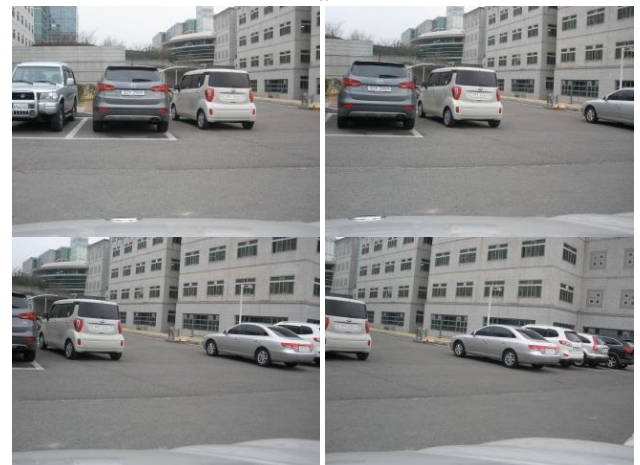
Fig. 6. Test image sets. (a) first row shows rotated image by every 10 degree increment angle to left direction out of 0 degree (i.e., L10, L20, L30, L40) and (b) second row shows rotated images by every 10 degree increment angle to right direction from 0 degree (i.e., R10, R20, R30, R40 degree). 0 degree image is referred as Fig. 4 - b).
