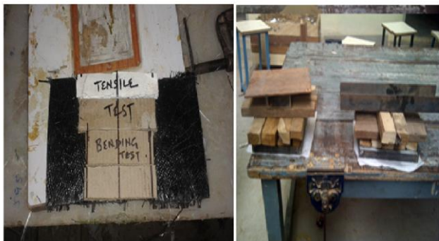
Fig.5. Preparation of Composite specimen for tensile and flexural testing.
