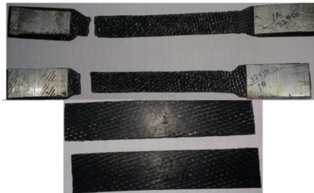
Fig. 9. Z-pinned carbon fiber laminates after performing tensile and bending test
