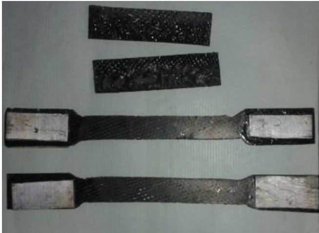
Fig.8. Z-pinned carbon fiber laminates before performing tensile and bending test
