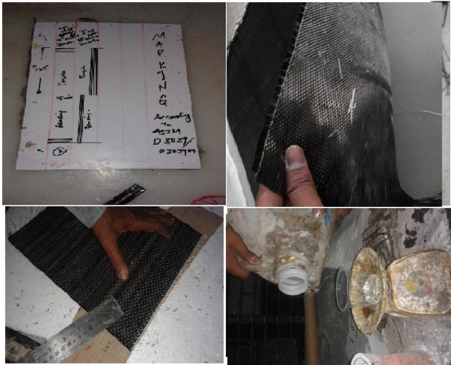
Fig.4. Preparation of Composite specimens
