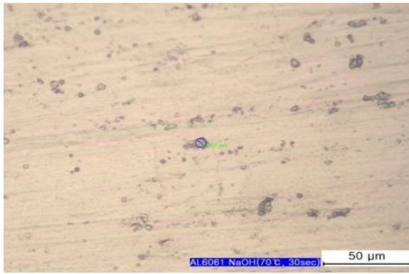
(c) After etching (NaOH)
