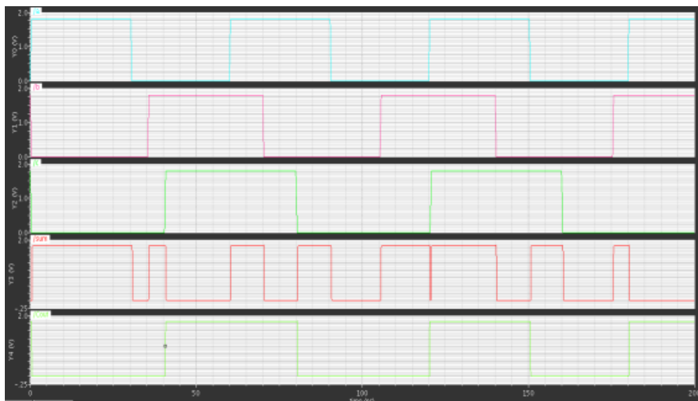
Fig:17 Conventional cmos full adder wave form
