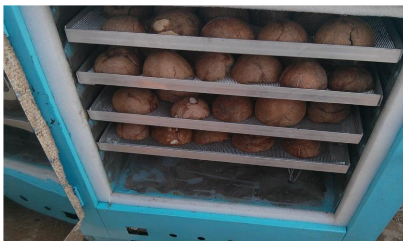
Figure – 2 Drying of Copra in the Cabinet Dryer
