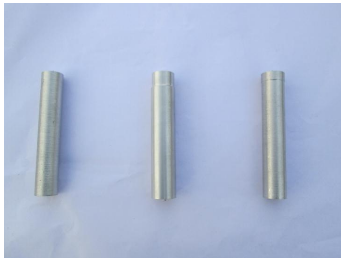
Figure 3: Photomicrograph of the Hybrid Composite Specimens after Turning operation
