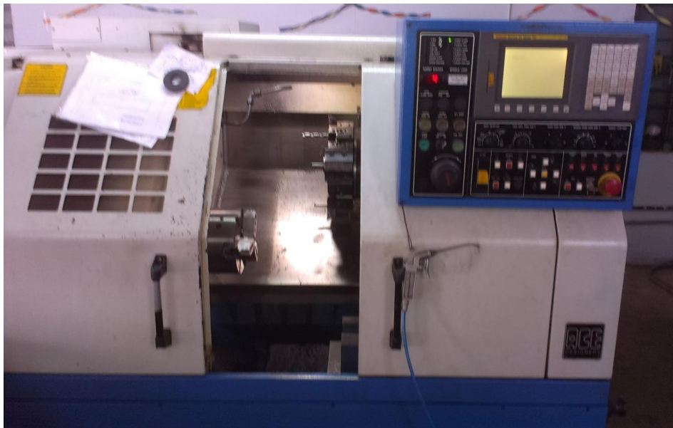
Figure 2: Experimental setup for Turning Hybrid Composites using CNC Lathe
