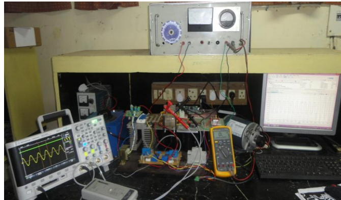
Figure 14. Full hardware setup of z source inverter with induction motor
