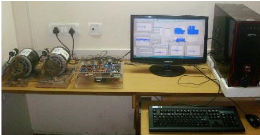
Fig. 8 Experimental setup using healthy and unhealthy motor
