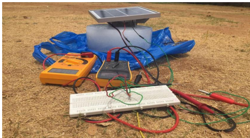
Figure.4.3. Solar panel with TEG with ICE cooling
