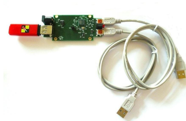
Figure 4: The USB switch with the switch-controlled PCDST SHIPKA
