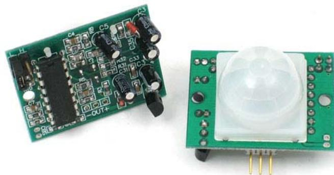
Fig. 2: Basic PIR Sensor
