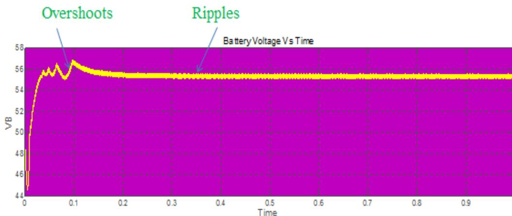
**Figure 8:** Voltage waveform of charging of 48 volt EV battery using PI controller
