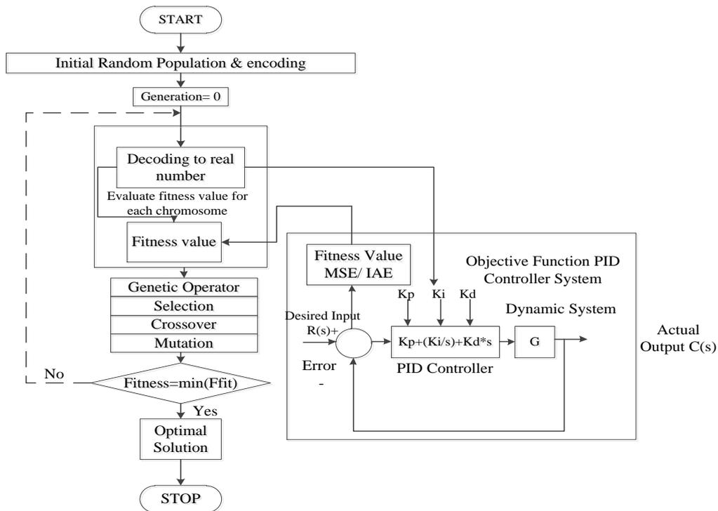
**Figure 6:** Flow chart implementation of GA-PID controller tuning
