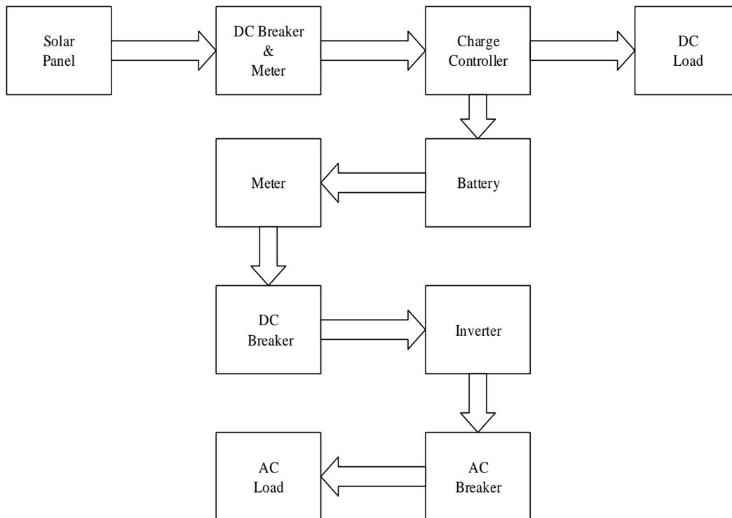
**Figure 13:** Standalone PV system design
