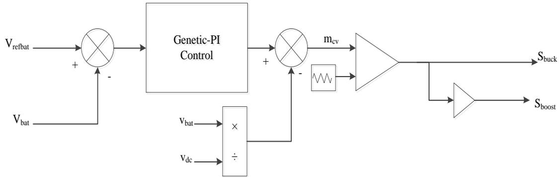
**Figure 5:** Constant voltage charging using Genetic control technique
