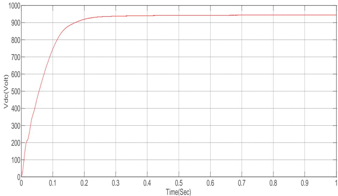
**Figure 12:** Variation of the DC bus voltage with respect to time.
