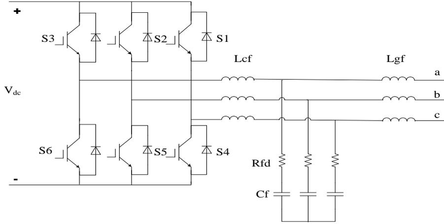
**Figure 1:** Three phase converter with passive LCL filter [17–18].
