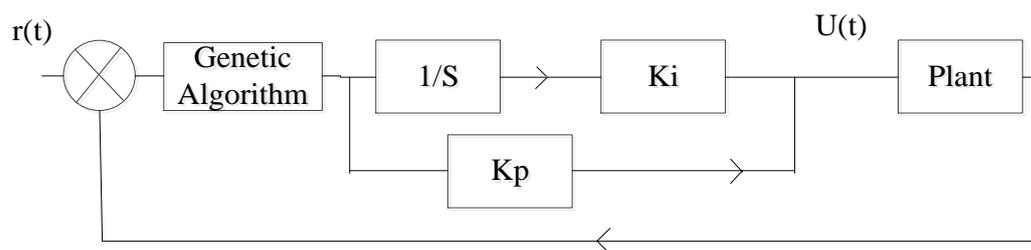
**Figure 7:** Block diagram of the GA-PI controller.
