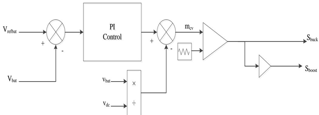
**Figure 4:** Constant voltage charging using PI control technique
