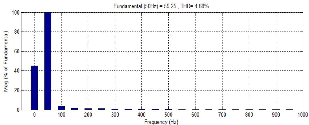
**Figure 10:** Current harmonics spectrum of 48 volt EV battery using PI controller
