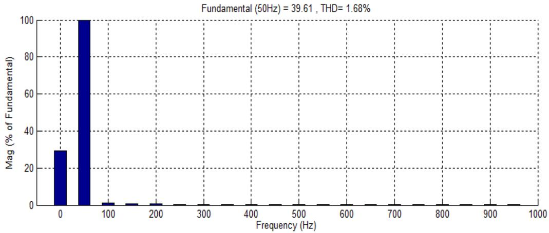
**Figure 11:** Current harmonics spectrum of 48 volt EV battery using GA-PI controller
