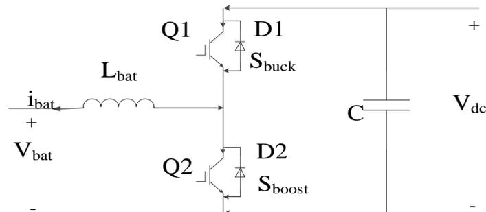
**Figure 2:** Half-bridge DC-DC converter
