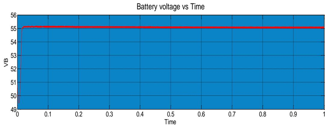
**Figure 9 :** Voltage waveform of charging of 48 volt EV battery using GA-PI controller.
