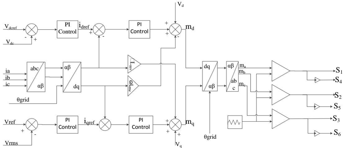
**Figure 3:** Control scheme of the charging station
